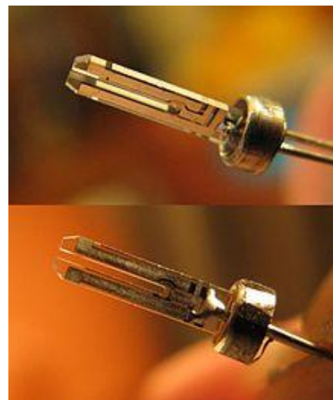
Picture of a quartz crystal resonator, used as the timekeeping component in quartz watches and clocks, with the case removed. It is formed in the shape of a tuning fork. Most such quartz clock crystals vibrate at a frequency of 32,768 Hz.
